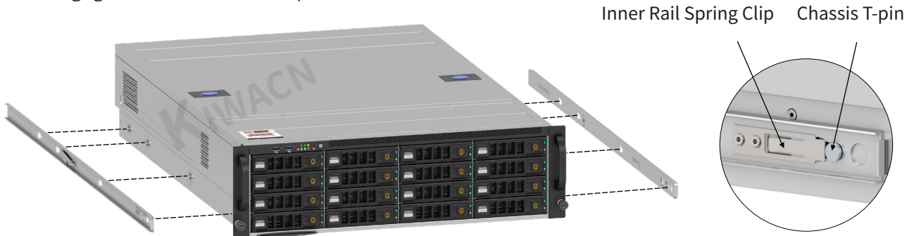
The inner rail spring clip engages with the chassis T-pin.
