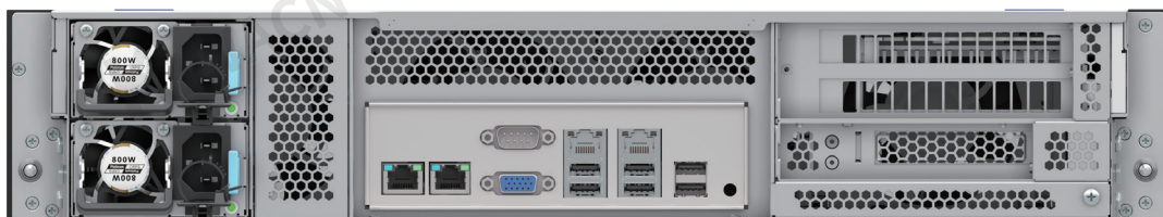
⑲ PCIe Installation Module (Motherboard Slot 2 Horizontal Rotation) Supports 16x Full-Height PCIe and 8x Half-Height PCIe
